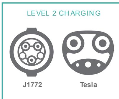
**Level 2 Charging:** Charging a vehicle at "Level 2" means plugging an EV into a 240 volt AC charger. The most common applications for Level 2 charging are at home or work and Level 2 chargers are also common in public areas such as public parking lots, hotels, restaurants and retail areas where EV drivers charge while engaged in other activities. On average, full charging time varies from 2 to 6 hours, but times vary by model and state of charge. Level 2 chargers use
