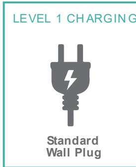
**Level 1 Charging:** Level 1 chargers plug directly into a standard 120 volt (V) AC outlet supplying an average power output of 1.3 kW to 2.4 kW. This power output is equivalent to 3-5 miles of EV range per hour. Level 1 charging uses standard NEMA 5-15 or NEMA 5-20 plugs. On average, full charging time varies and can take up to 20 hours, but times vary by model and state of charge.
